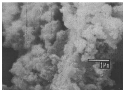
Fig. 1a SEM micrograph of \gamma -Fe 2 O 3 prepared from ferrous hydroxide precursor (NM 1 )
